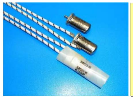
Example: **3HM525-36** Bimetal of 35ohms/cmf, Operating temperature 170°C, Reset temperature 92°C, with #6 heater, High capacity contacts (80A), DMD-wire leads AWG#14, 240mm (Can side) length and 190mm (Pin side) length with strip length 10mm, Insulation sleeve by Toray Lummror X10S, 55mm length
