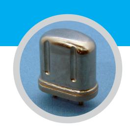
PRODUCT OVERVIEW The Klixon® 34HM on-winding motor protector is a 3-phase line break, automatic reset device which interrupts line current at the centerpoint of a WYE (Star) wound motor.
